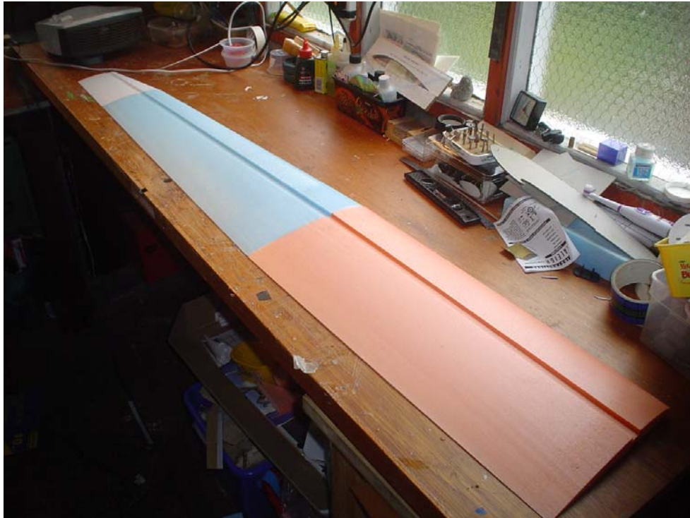
The 3 panels of the left wing with the groove cut for the carbon tow spar
